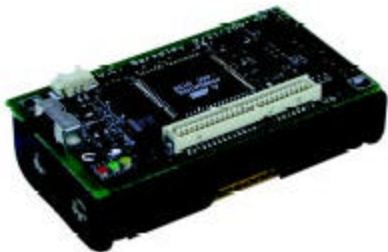
Figure 1 – A Berkeley field-node (mote)
